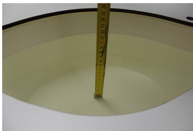
Liquid depth in the Body Phantom (1900 MHz 15cm depth)
