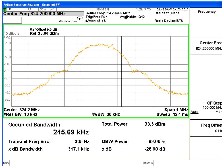
Occupied Bandwidth (99%) GPRS 850 BAND CH 190
