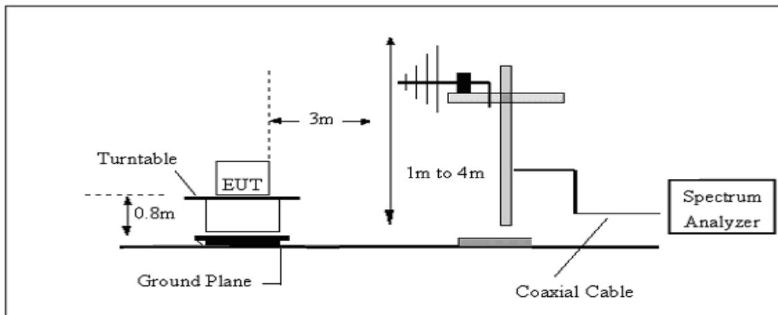
(B) Radiated Emission Test-Up Frequency Above 1GHz
