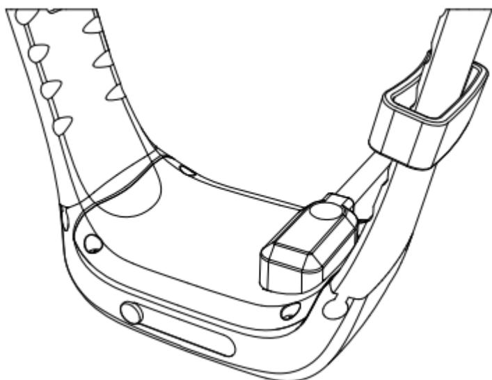
Connect one end of the charging cable to the charger of 5V output power that conforms to the national standard , or to USB interface on computer, mobile power charger, etc., then charge in a dry environment making sure that the magnetic suction charger and watch charging interface are coincided each other. **Slight heat releasing from device** in charging process belongs to the normal phenomenon. Generally battery can be filled with 2-3 hours charging.
