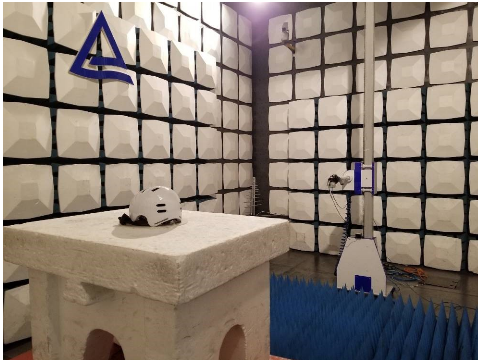
Photograph 4: Set-up for Radiated Spurious Emission, 18GHz - 26.5GHz
