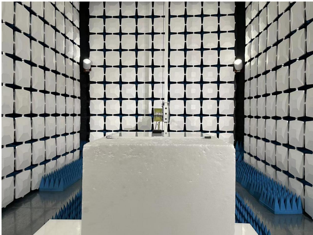
Above 1GHz for radiated emission test setup
