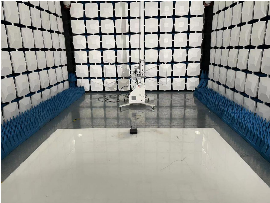
Above 1GHz for radiated emission test setup
