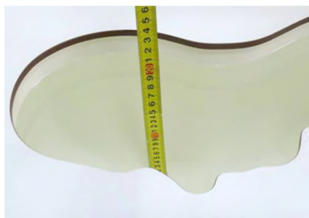
Liquid depth in the head phantom (835MHz)
