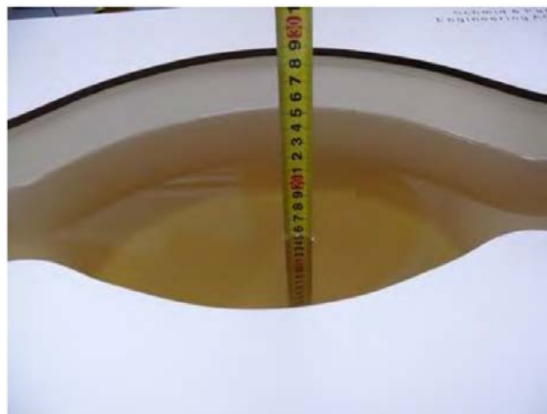
Liquid depth in the body phantom (835MHz)
