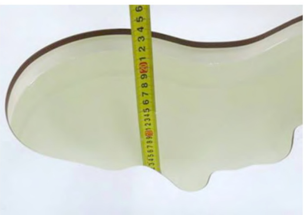
Liquid depth in the head phantom (1900MHz)
