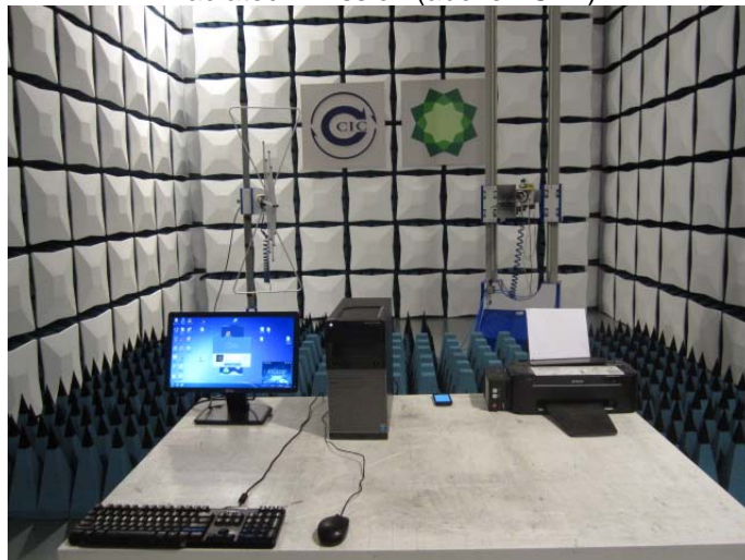
Radiated Emission (above 1GHz)
