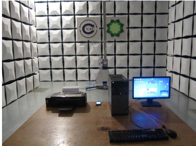
Radiated Emission (above 1GHz)
