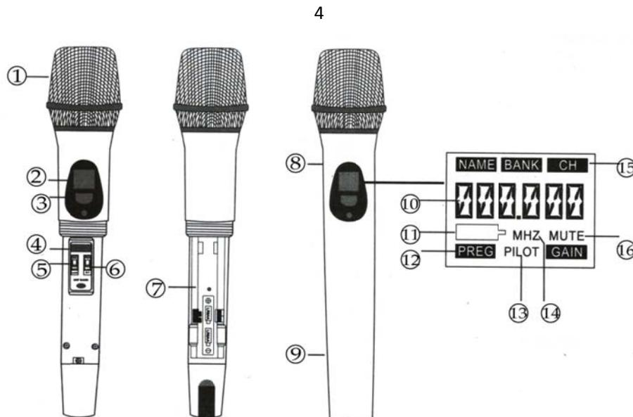
① Microphone head: including head and sound modules.
