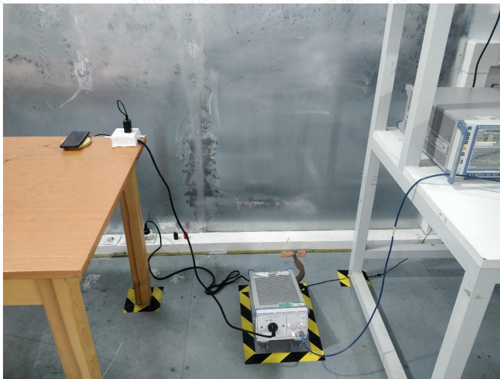
Conducted Emission-AC adapter charge mode
