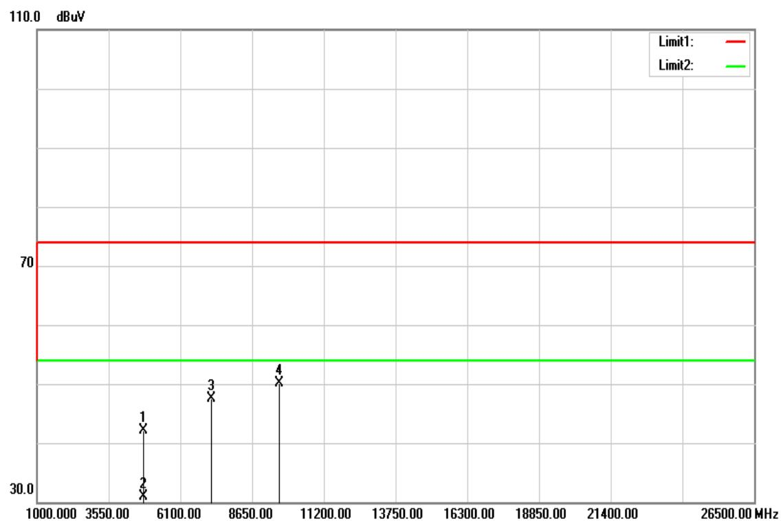
**Above 1 GHz****Operation Mode:** GFSK / TX / CH Low**Test Date:** March 25, 2016**Temperature:** 27°C**Tested by:** Jason Lu**Humidity:** 53 % RH**Polarity:** Ver. / Hor.
