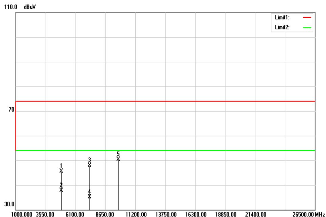
**Operation Mode:** TX / IEEE 802.11b / CH Mid**Test Date:** March 25, 2016**Temperature:** 27°C**Tested by:** Jason Lu**Humidity:** 53% RH**Polarity:** Ver. / Hor.
