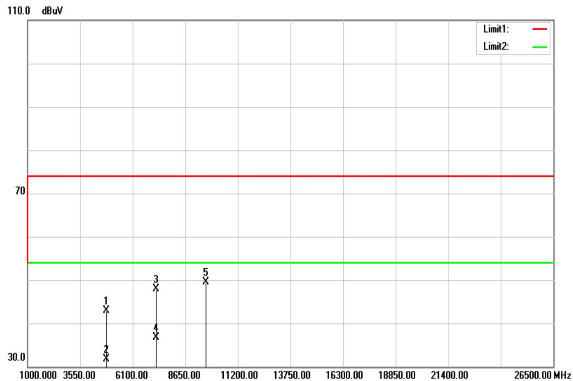
**Operation Mode:** TX / IEEE 802.11g / CH High**Test Date:** March 25, 2016**Temperature:** 27°C**Tested by:** Jason Lu**Humidity:** 53% RH**Polarity:** Ver. / Hor.
