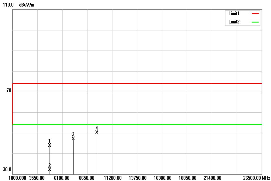
**Above 1 GHz****Operation Mode:** TX / IEEE 802.11b / CH Low**Test Date:** February 26, 2016**Temperature:** 27°C**Tested by:** Jason Lu**Humidity:** 53% RH**Polarity:** Ver. / Hor.
