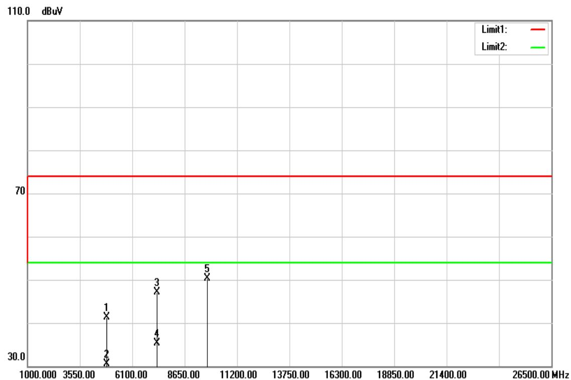
**Operation Mode:** TX / IEEE 802.11g / CH Mid**Test Date:** March 25, 2016**Temperature:** 27°C**Tested by:** Jason Lu**Humidity:** 53% RH**Polarity:** Ver. / Hor.
