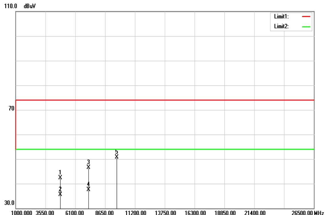
**Operation Mode:** TX / IEEE 802.11g / CH Low**Test Date:** March 25, 2016**Temperature:** 27°C**Tested by:** Jason Lu**Humidity:** 53% RH**Polarity:** Ver. / Hor.
