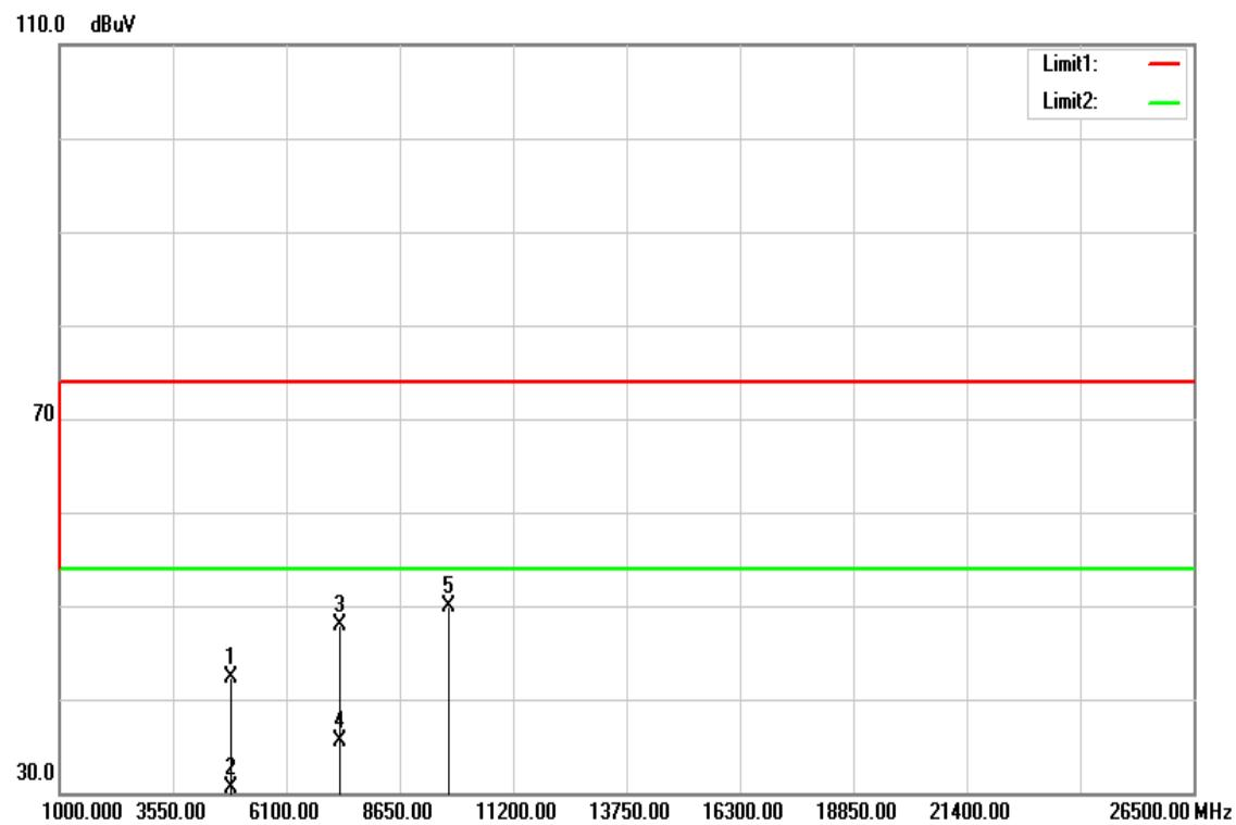
**Operation Mode:** TX / IEEE 802.11n HT 20 MHz mode / CH Mid **Test Date:** March 25, 2016**Temperature:** 27°C**Tested by:** Jason Lu**Humidity:** 53% RH**Polarity:** Ver. / Hor.
