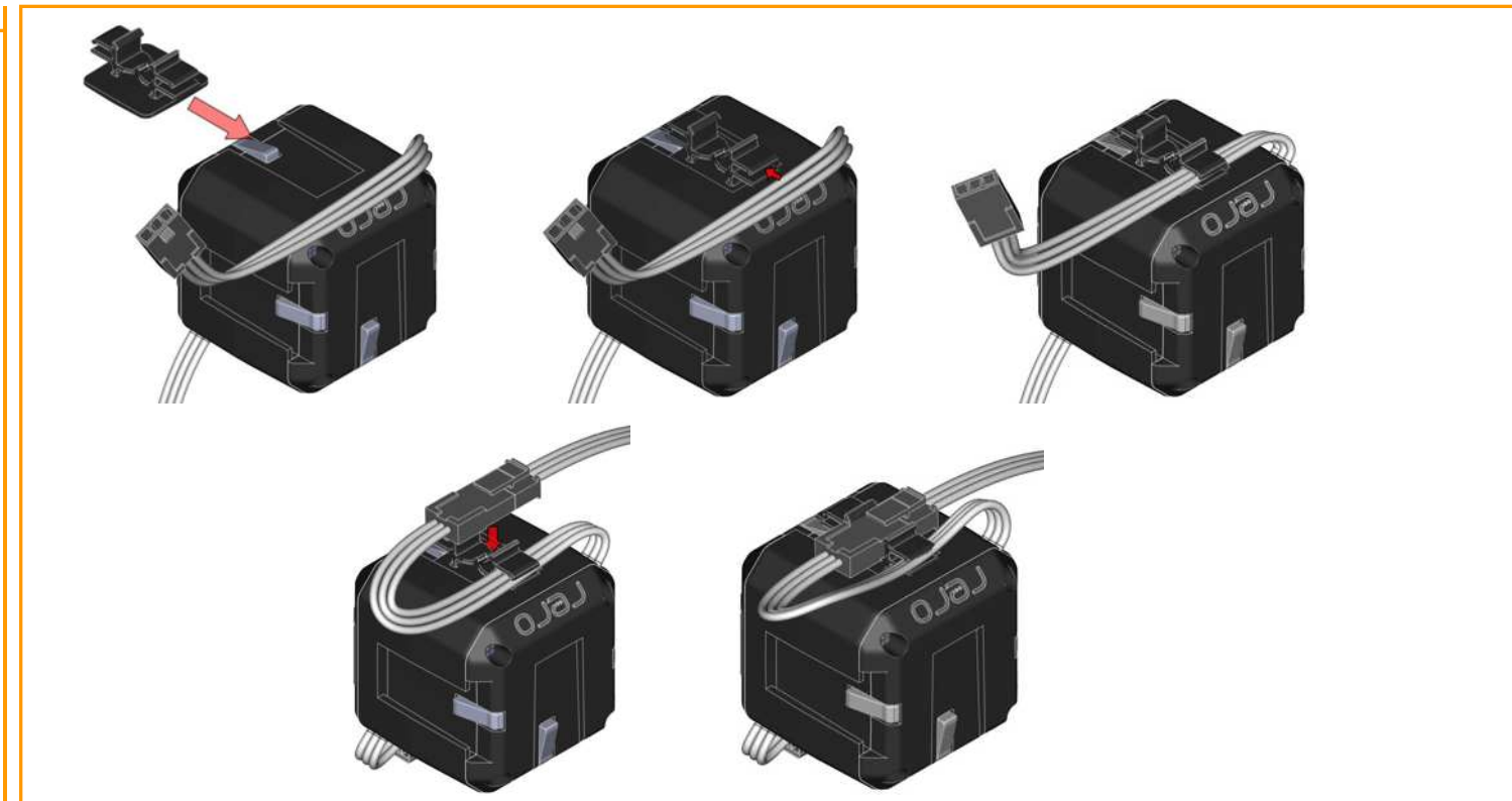
Organizing wires and connectors using wire clip
