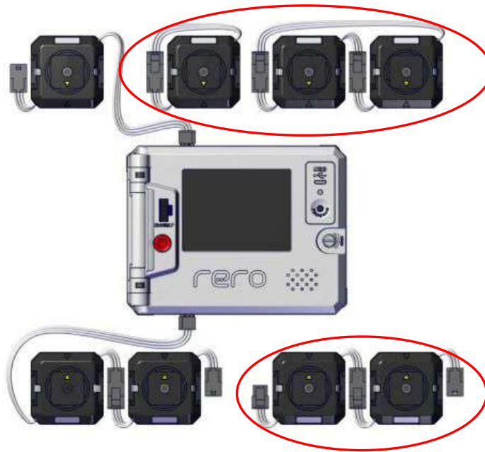
Wrong or Broken Daisy Connection
