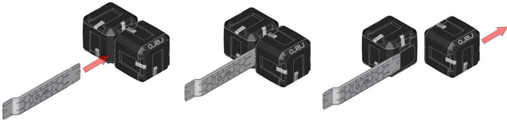
Release rero Cube joint from Interconnect
