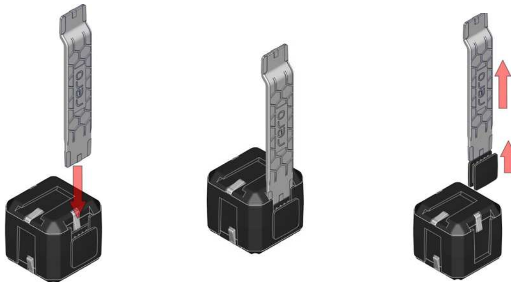
Release rero Interconnect from Cube Joint slot
