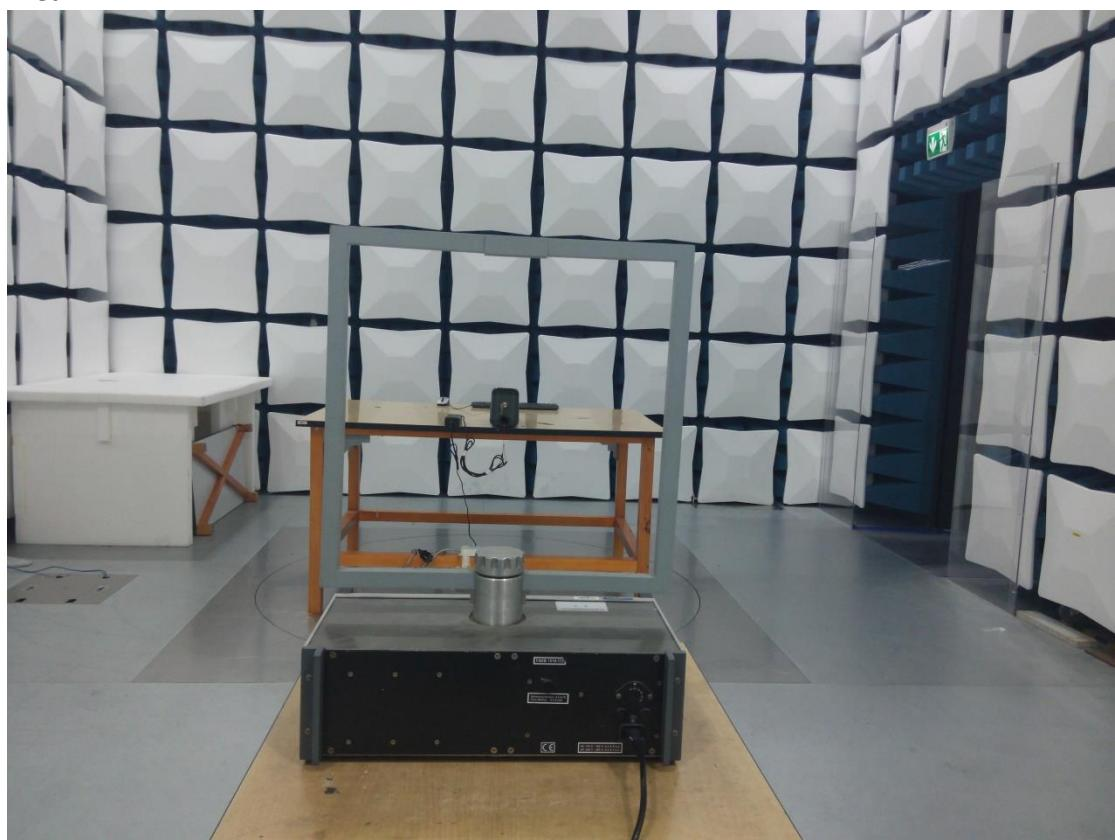
FCC Part15C Radiated Emission below 1GHz
