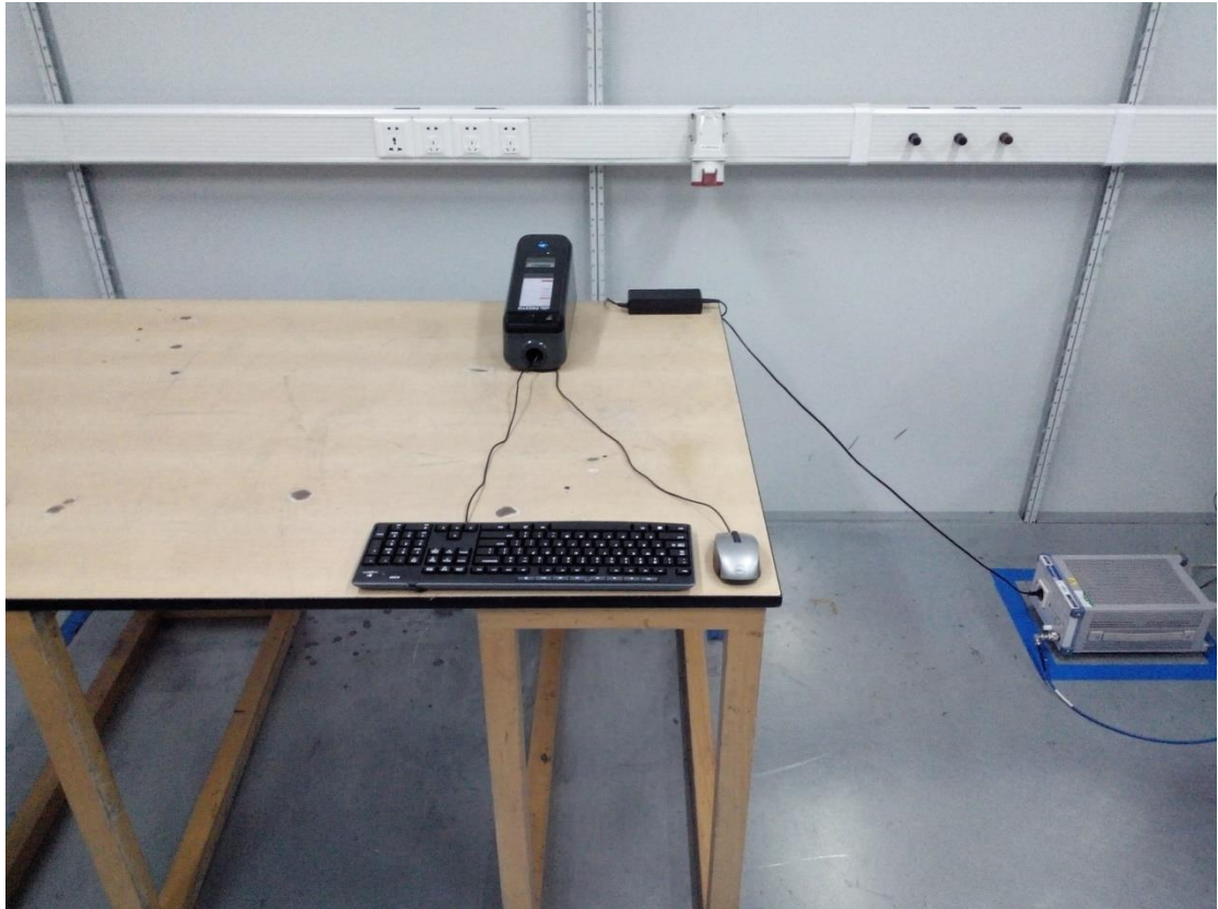
AC Conducted Emission Test Setup -Front
