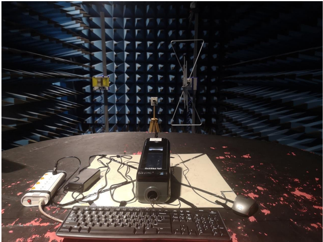
FCC Part15E Radiated Emission above 18-26.5GHz
