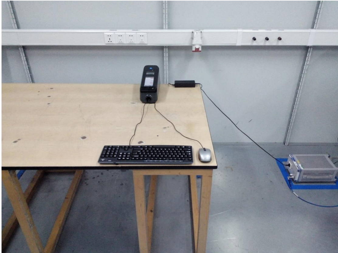
AC Conducted Emission Test Setup -Front
