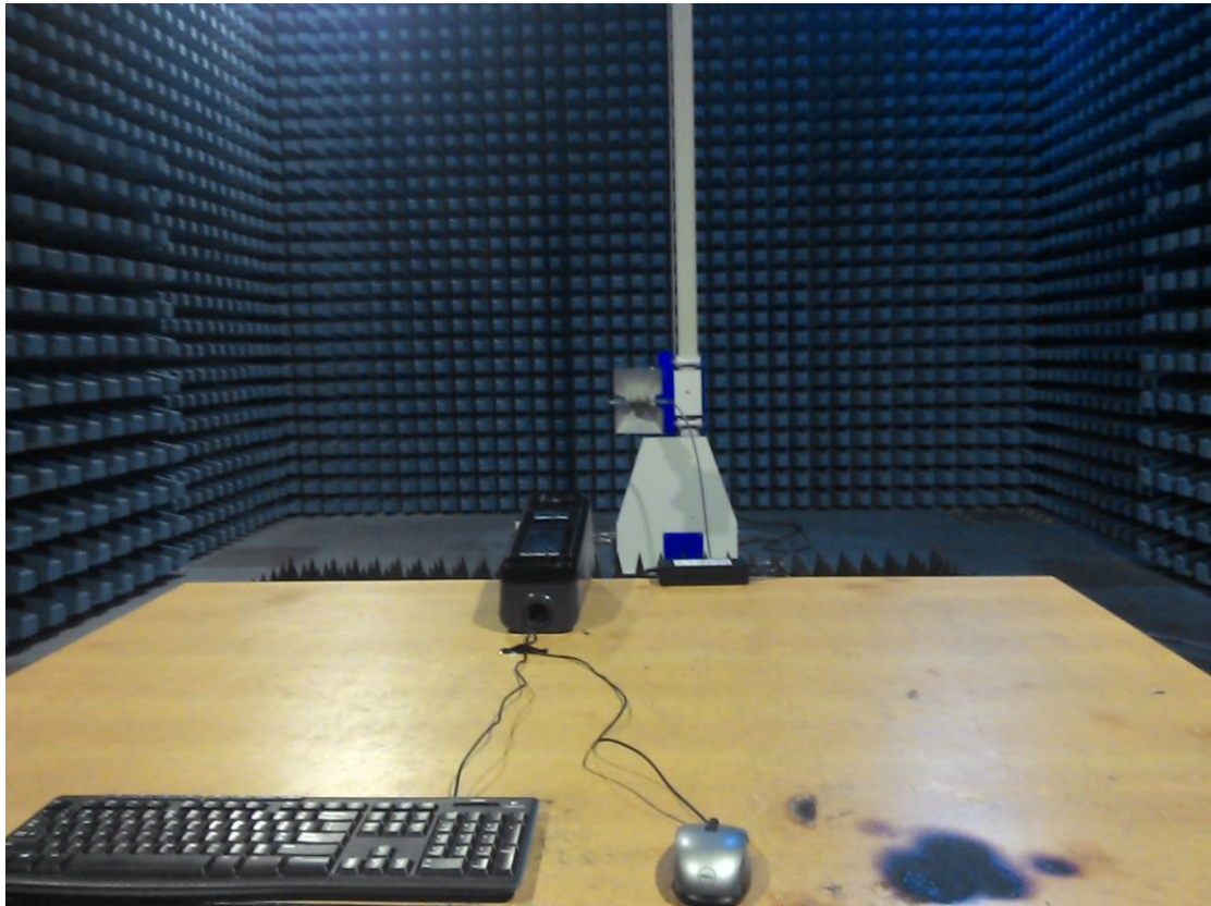
FCC Part15B Radiated Emission above 1GHz -Front
