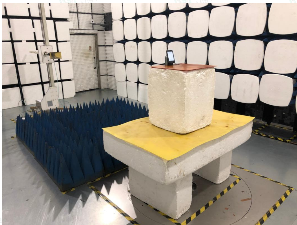
Radiated Emissions Measurement (Above 1GHz)
