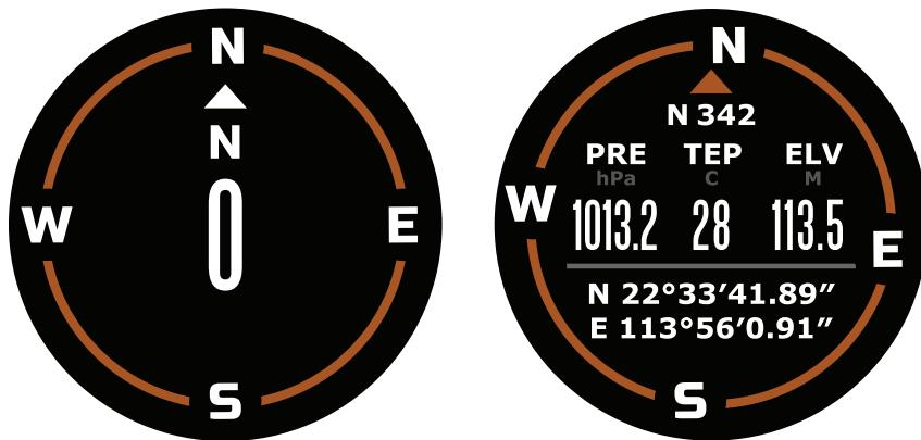
Select START button or slide from right to left on the screen, enter the details interface, you can see the information for air pressure, temperature(obtained from the built-in thermometer), altitude and coordinates.
