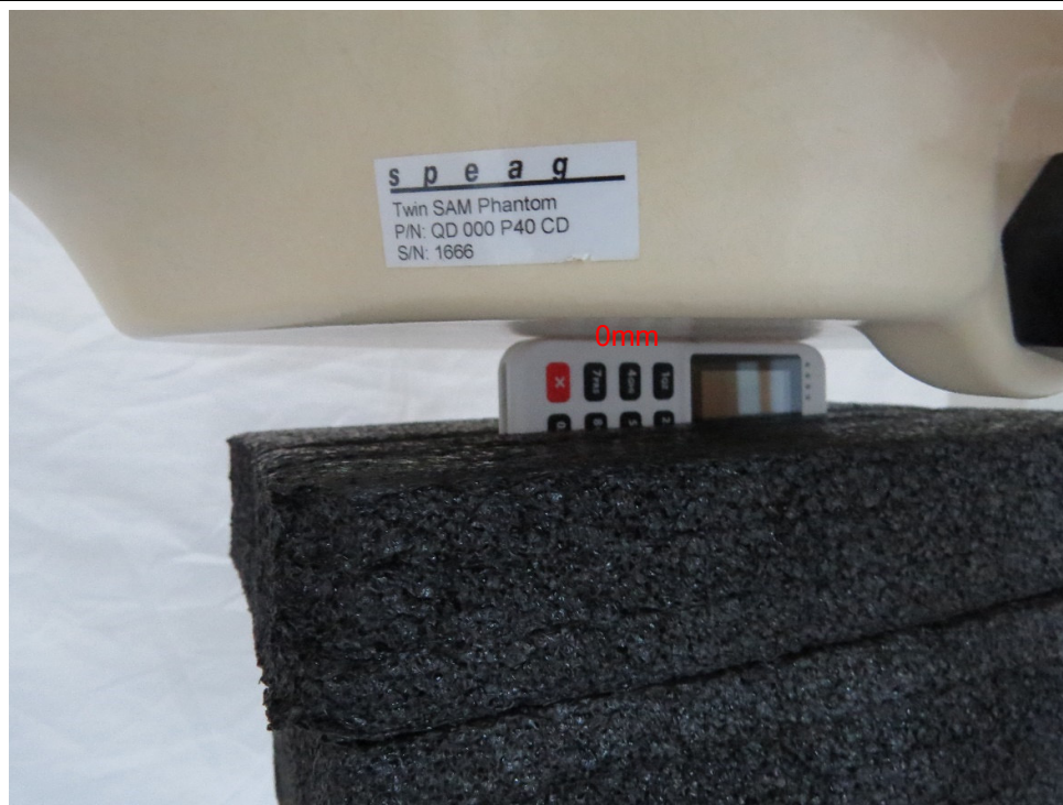
Picture 9: Left Edge, the distance from EUT to the bottom of the Phantom is 0mm
