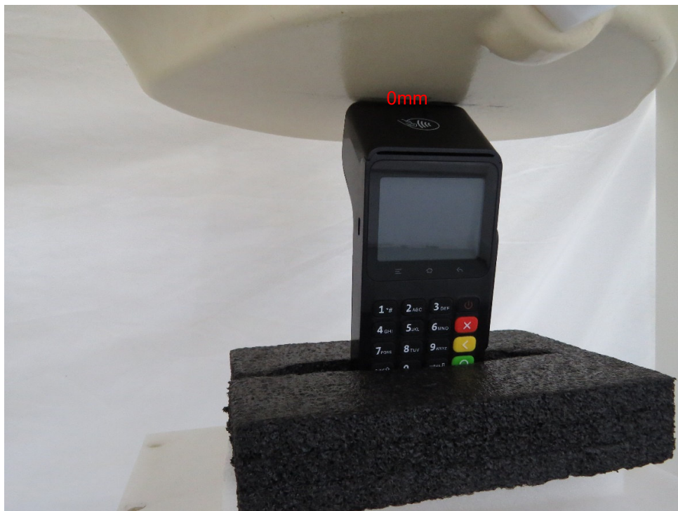
Picture 15: Top Edge, the distance from EUT to the bottom of the Phantom is 0mm
