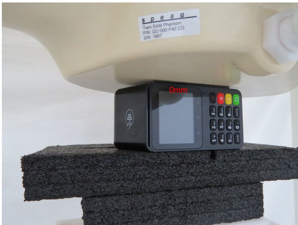
Picture 14: Right Edge, the distance from EUT to the bottom of the Phantom is 0mm
