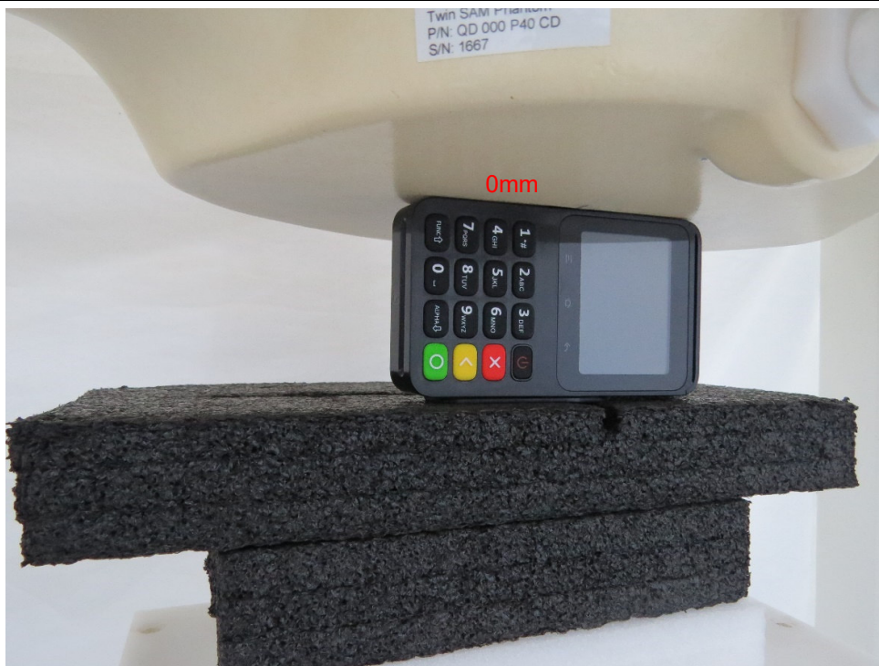
Picture 13: Left Edge, the distance from EUT to the bottom of the Phantom is 0mm
