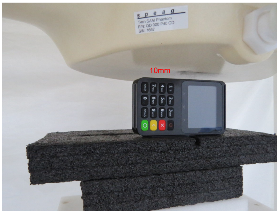
Picture 5: Left Edge, the distance from EUT to the bottom of the Phantom is 10mm
