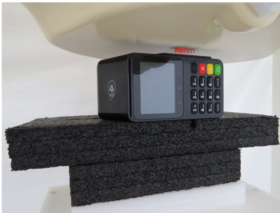
Picture 6: Right Edge, the distance from EUT to the bottom of the Phantom is 10mm
