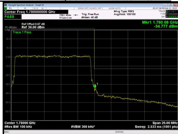
HLTE Band66 QAM64 BW=10MHz Channel=132622 RB Size=50 Position=#0
