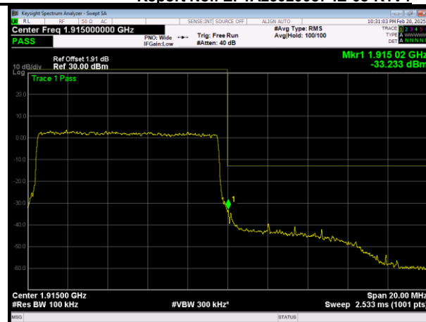
H\LTE Band25 QPSK BW=10MHz Channel=26640 RB Size=50 Position=#0
