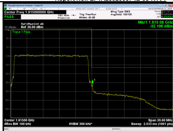
H\LTE Band25 QAM64 BW=10MHz Channel=26640 RB Size=50 Position=#0
