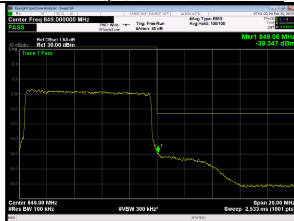
HLTE Band5 QAM16 BW=10MHz Channel=20600 RB RB Size=50 Position=#0
