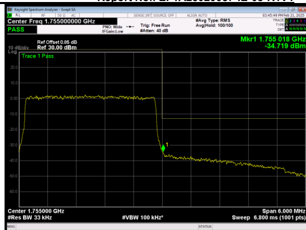
HLTE Band4 QAM64 BW=3MHz Channel=20385 RB Size=15 Position=#0
