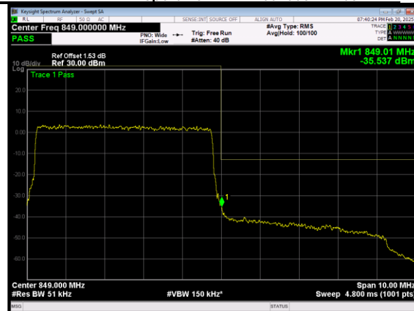
H\LTE Band5 QPSK BW=5MHz Channel=20625 RB Size=25 Position=#0
