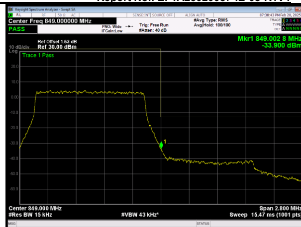
HLTE Band5 QPSK BW=1.4MHz Channel=20643 RB Size=6 Position=#0
