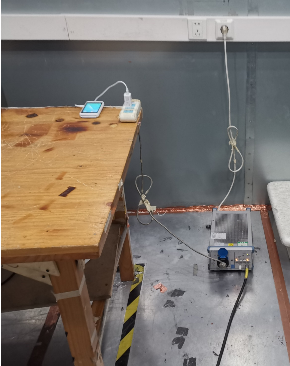
Picture 2: Conducted Emissions Test Setup
