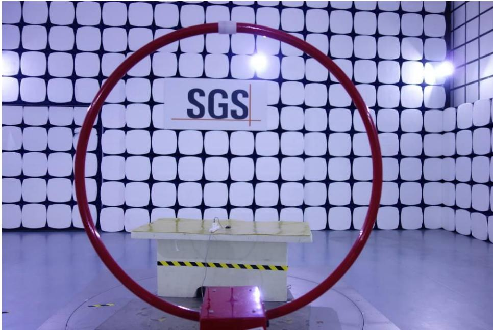
**1.4 Radiated Emissions(30MHz-1GHz) Test Setup**
