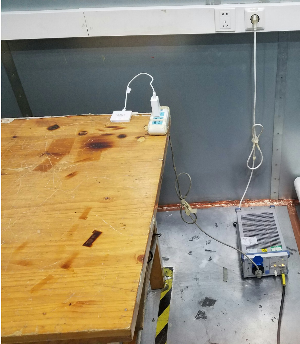
Picture 2: Conducted Emissions Test Setup
