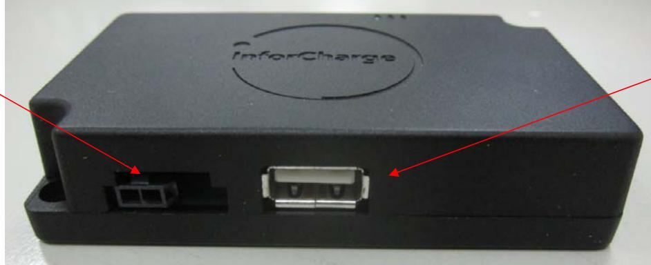
1. Can give control to 5V or 36V output to other devices, such as wireless charging equipment
