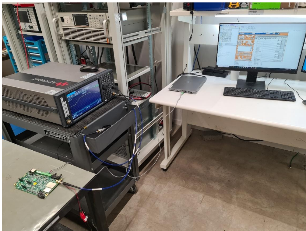
Conducted RF measurement setup
