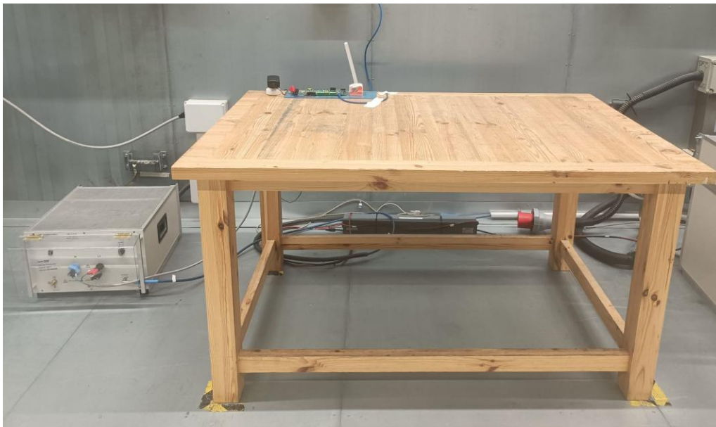
Conducted Emission measurement setup
