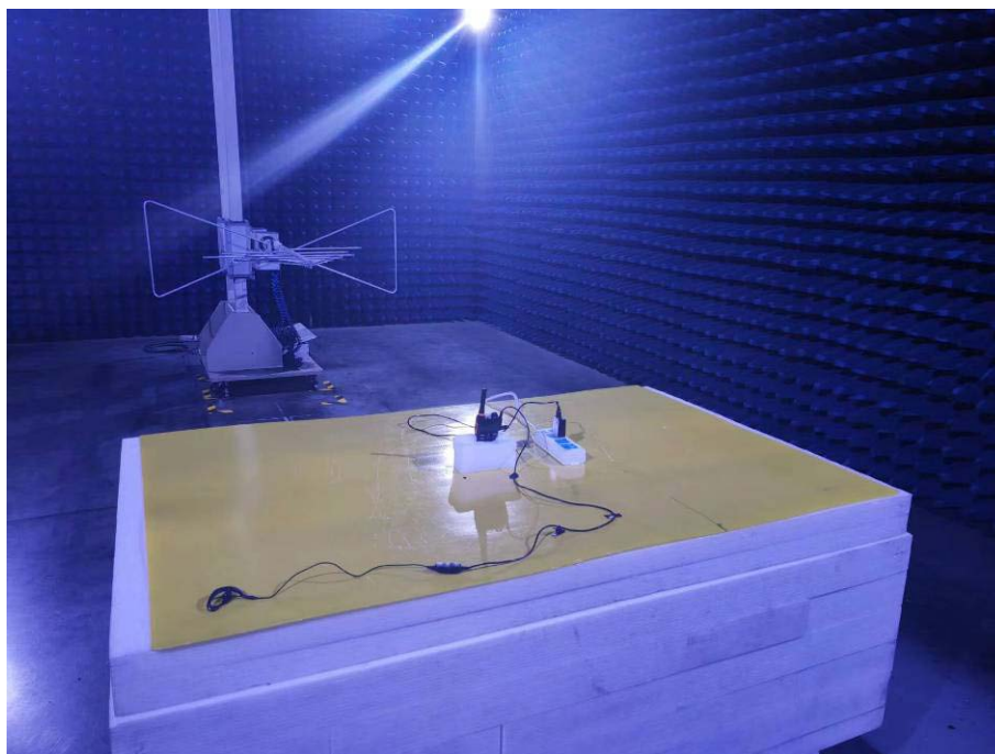
Photo of Radiated Emission Measurement Below 1GHz
