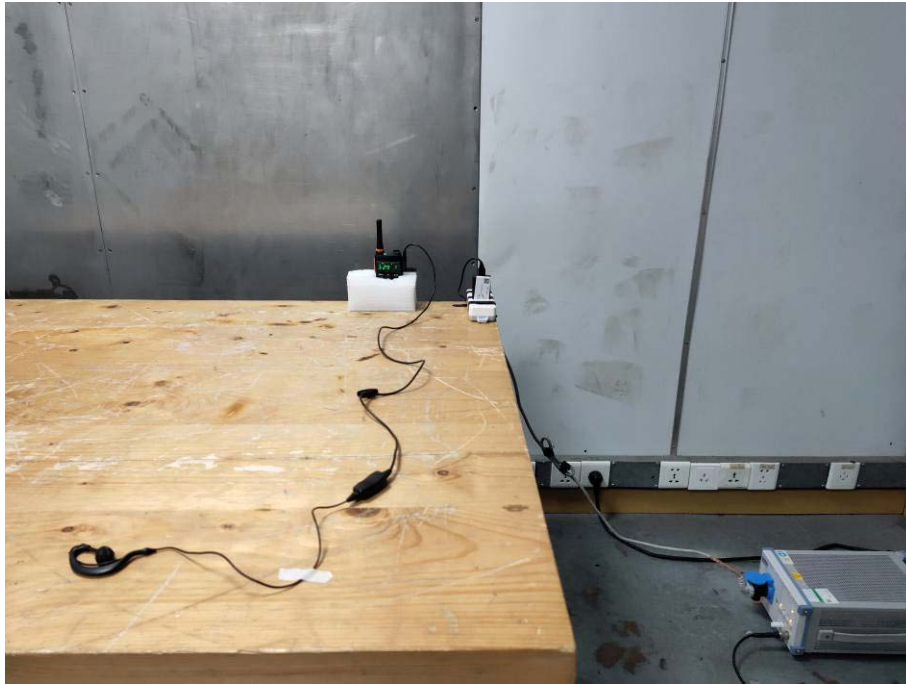
Photo of Conducted Emission Measurement
