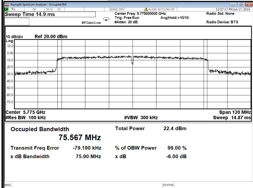
**IEEE 802.11ac 80 MHz mode / 5775MHz****6dB Bandwidth****Antenna 1**
