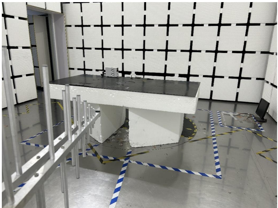
Radiation Emission Test Setup (30MHz to 1GHz)
