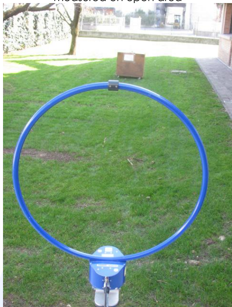
0,15 – 30 MHz radiated disturbance at 10 m distance measured on open area
