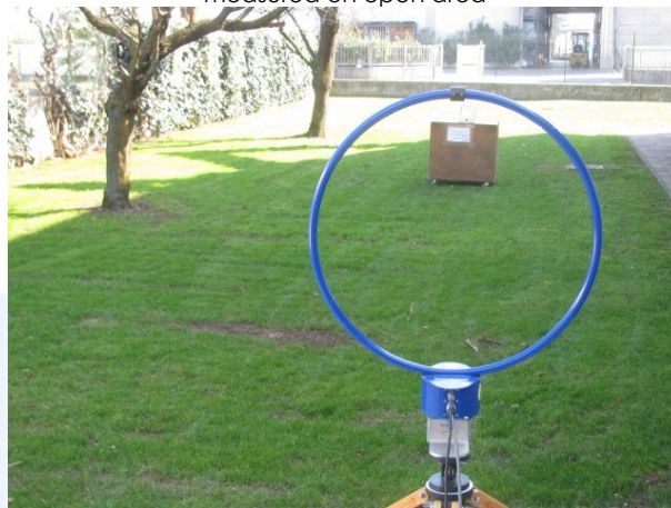
0,15 – 30 MHz radiated disturbance at 10 m distance measured on open area
