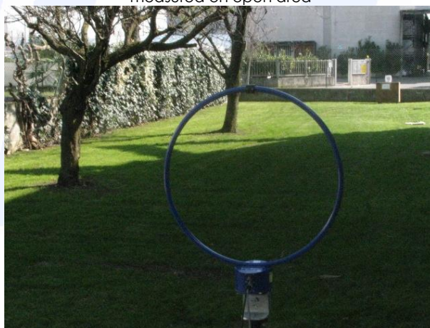
0,15 – 30 MHz radiated disturbance at 30 m distance measured on open area
