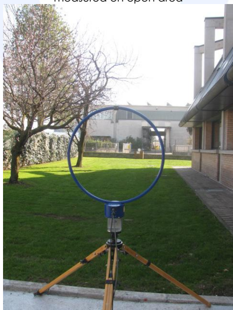
0,15 – 30 MHz radiated disturbance at 30 m distance measured on open area
