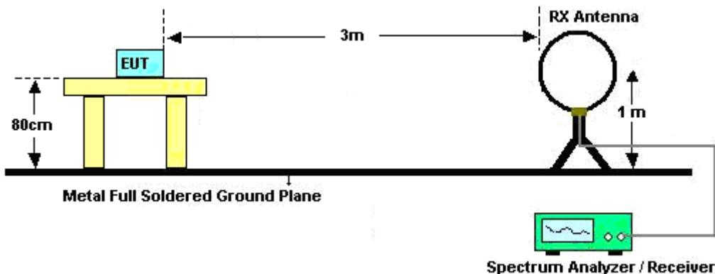
For radiated emissions from 30MHz to 1GHz
