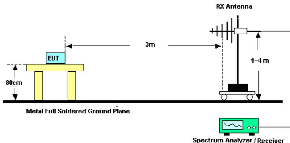
For radiated test from 1GHz to 18GHz
