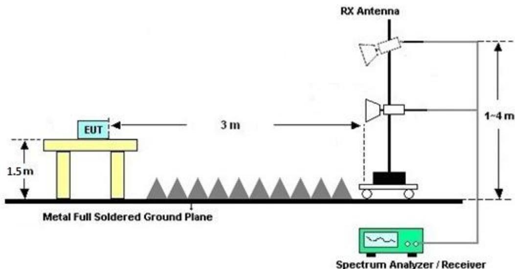
For radiated test above 18GHz
