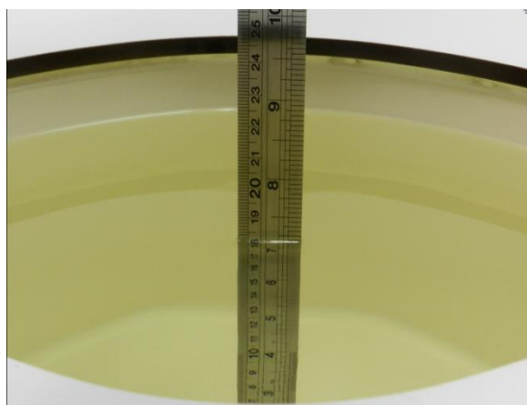
Fig 10.2 Photo of Liquid Height for Body SAR
