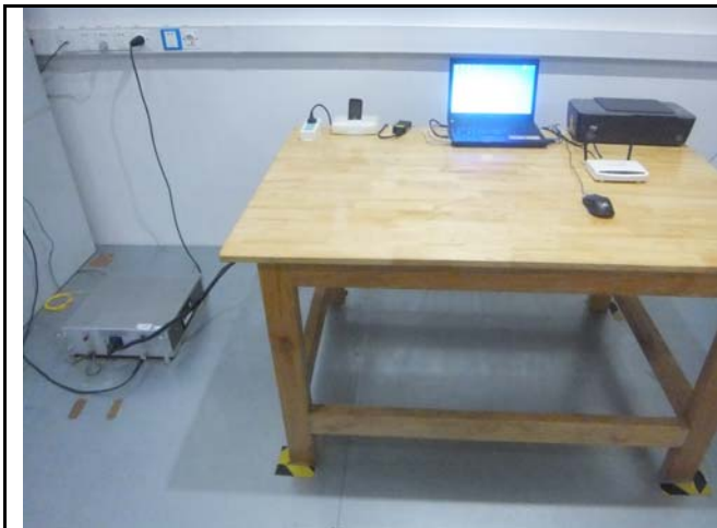
Conducted Emissions Test Setup – Front View
