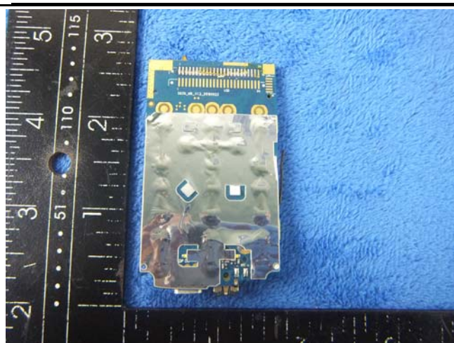
Mainboard with Shielding - Rear View
