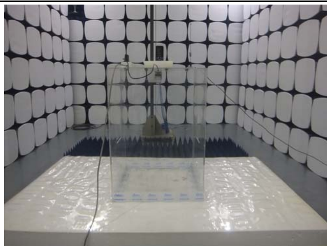
Radiated Spurious Emissions Test Setup Above 1GHz
