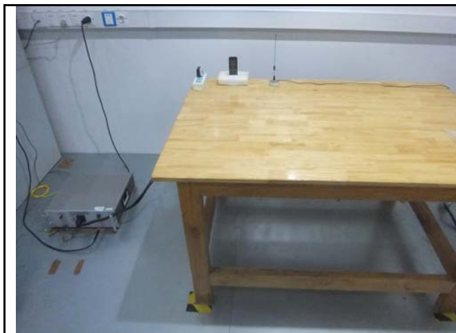
Conducted Emissions Test Setup Front View
