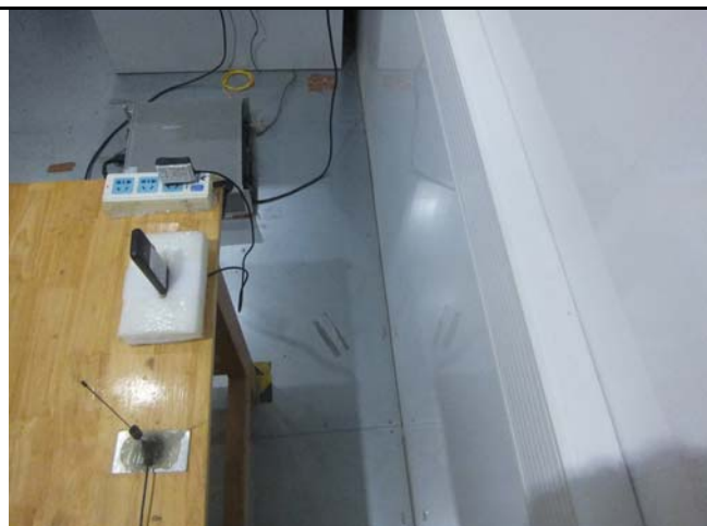
Conducted Emissions Test Setup Side View
