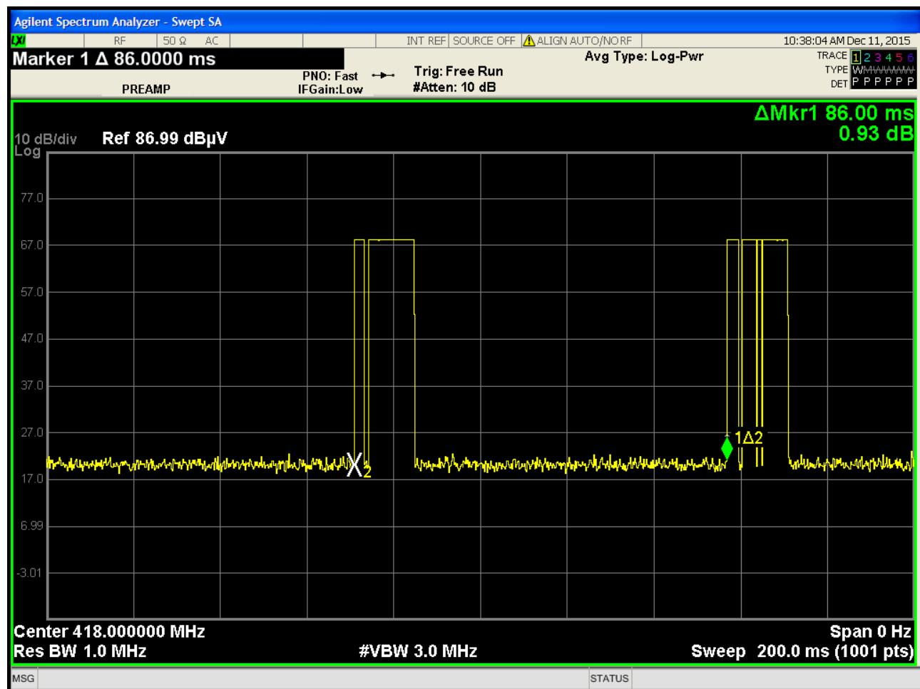
Total Pulse Time with Blanking Interval is 86.00 ms
