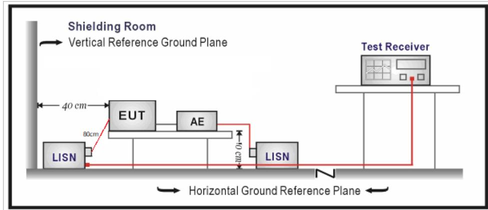
Note: AC Power source is used to change the voltage 110V/50Hz.
