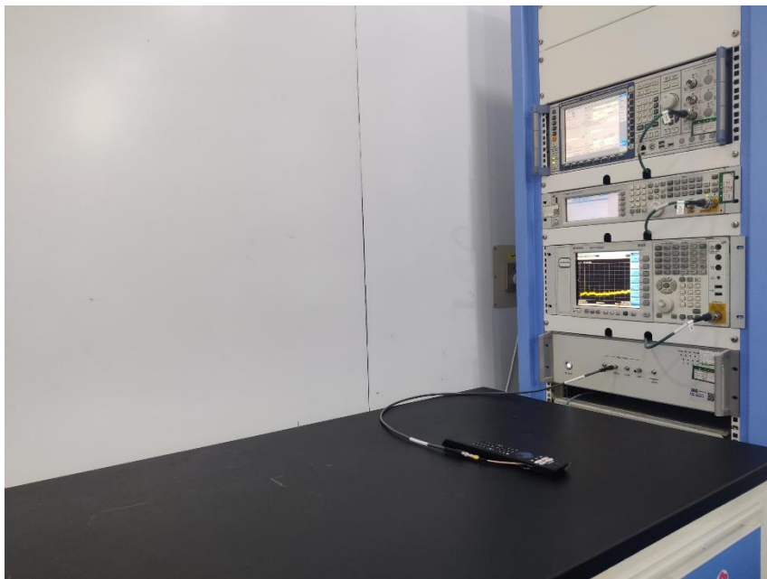
Conducted test setup
