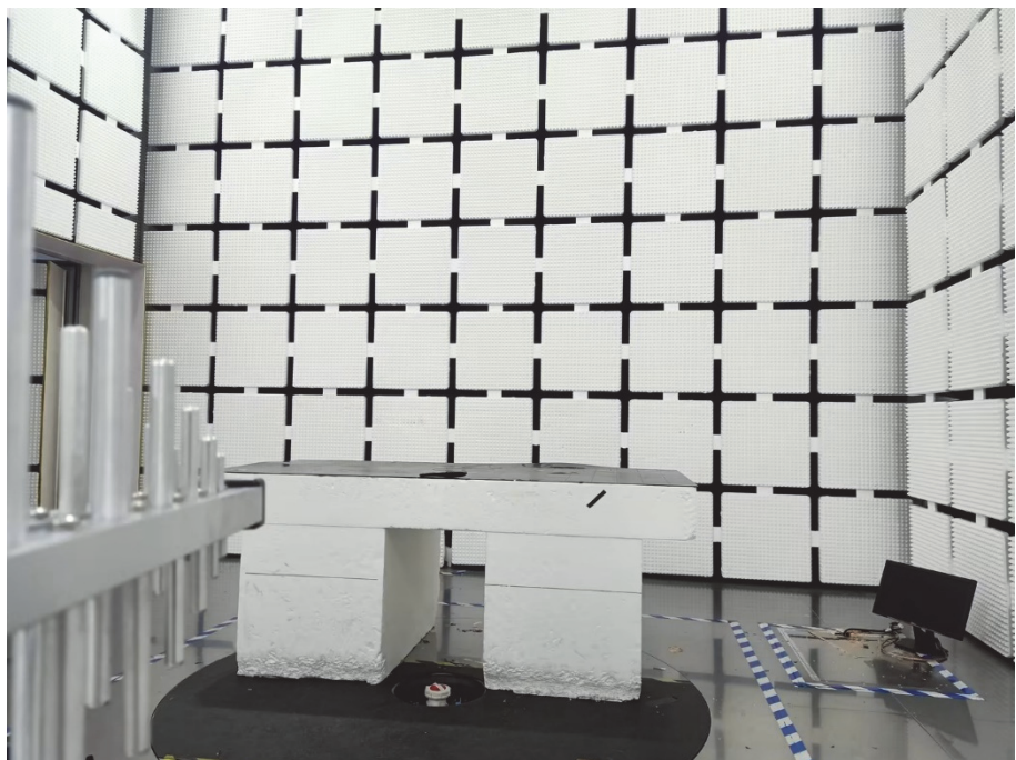
Radiation Emission Test Setup (30MHz to 1GHz)
