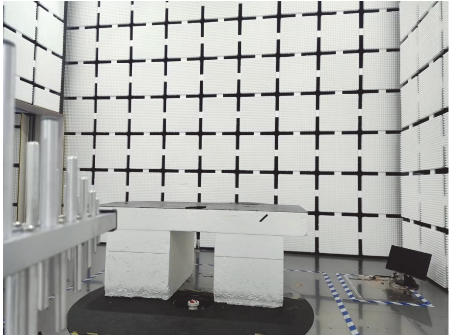
Radiation Emission Test View (30MHz to 1GHz)
