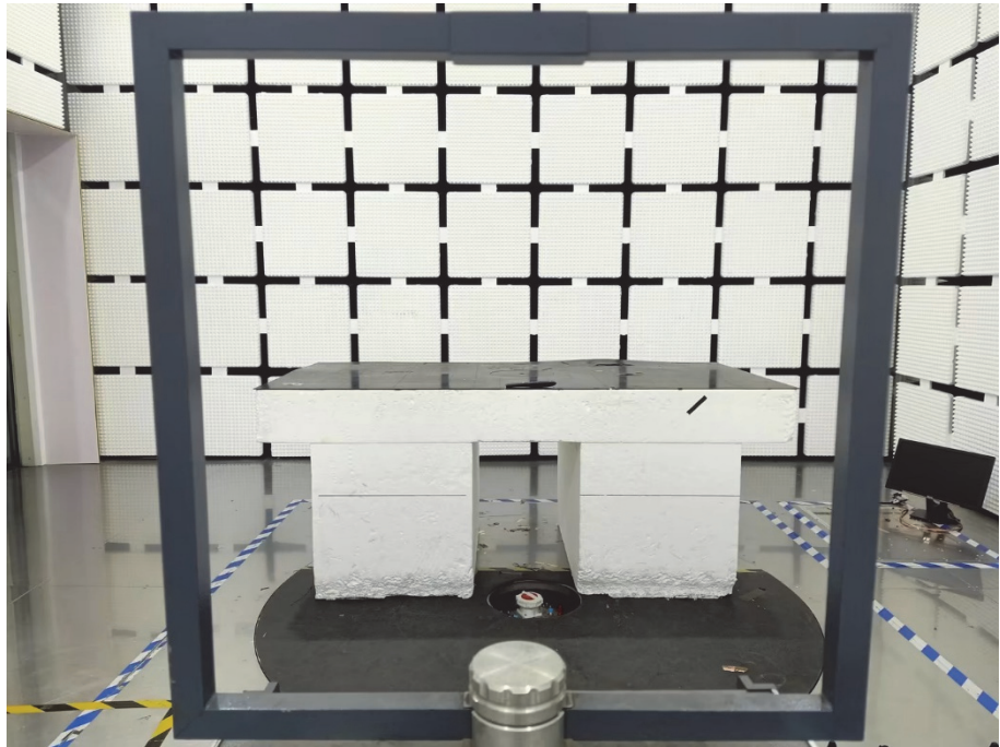
Radiation Emission Test Setup (Below 30MHz)
