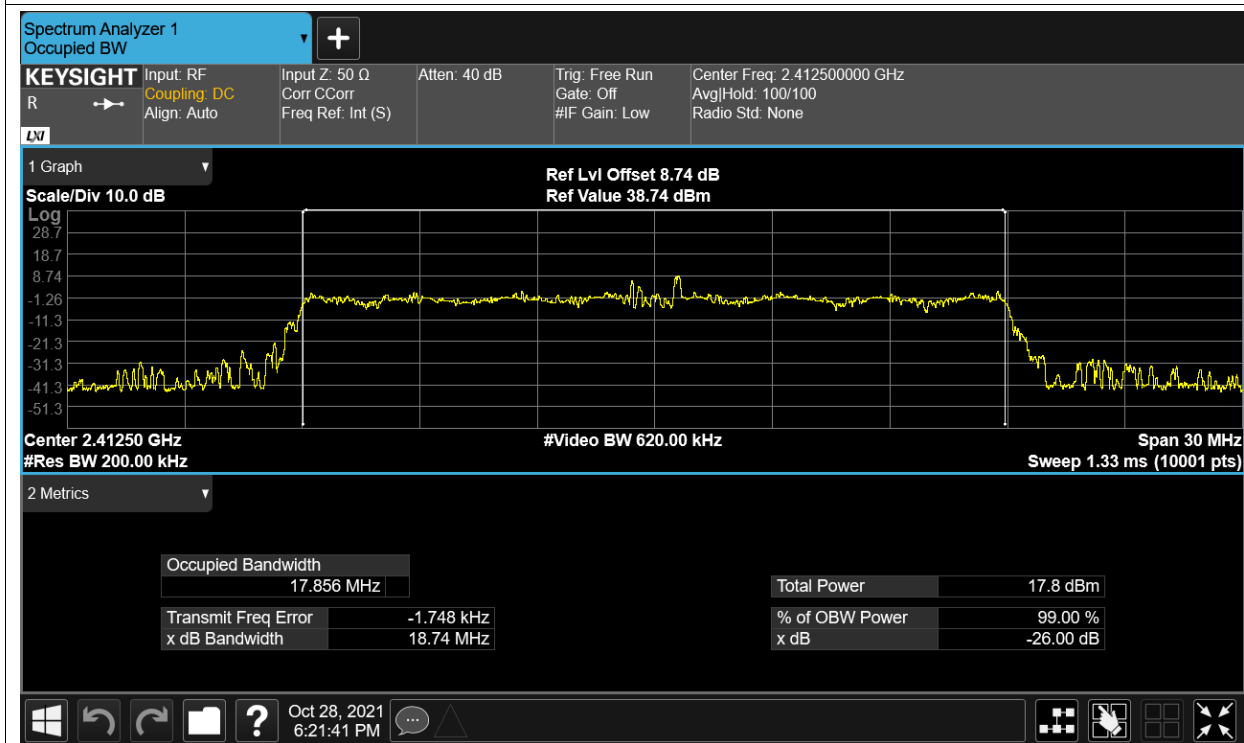
OBW NVNT 2.4G-20M-QPSK 2437.5MHz Ant1
