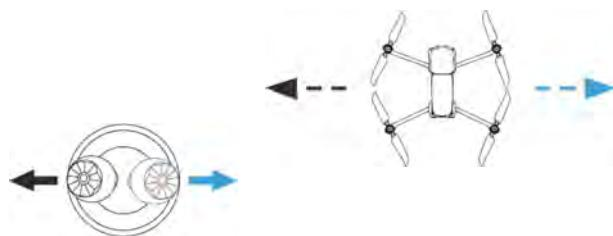
1. The left-and-right direction of the right stick is the roll stick, which is used to control the flight of the aircraft in the left and right directions.
