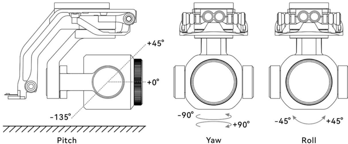
Fig 3-11 Mechanical Rotation Range of the Gimbal
