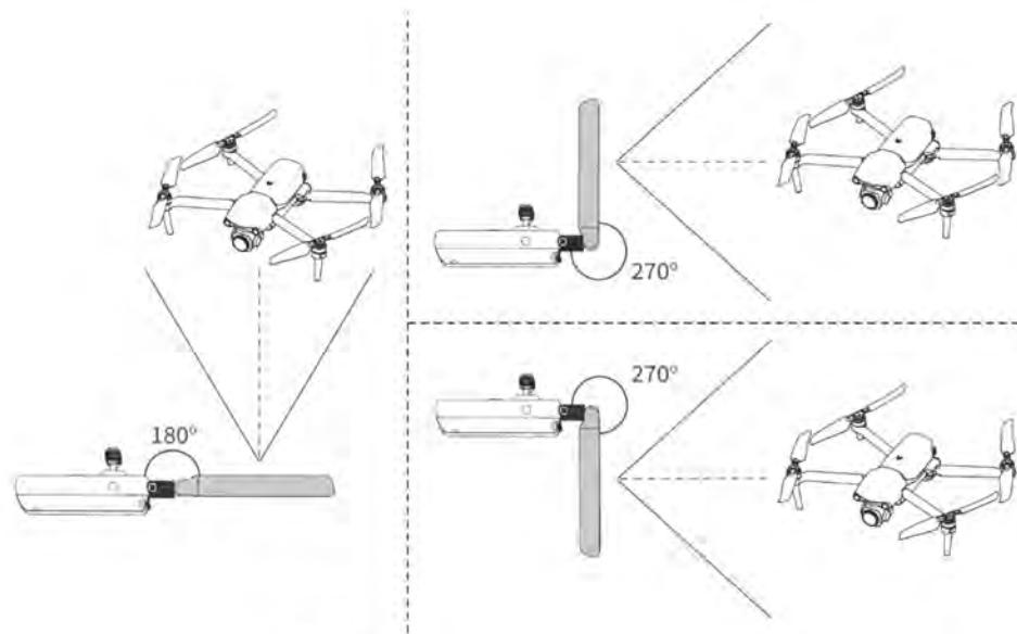
Fig 4-9 Extend the antenna
