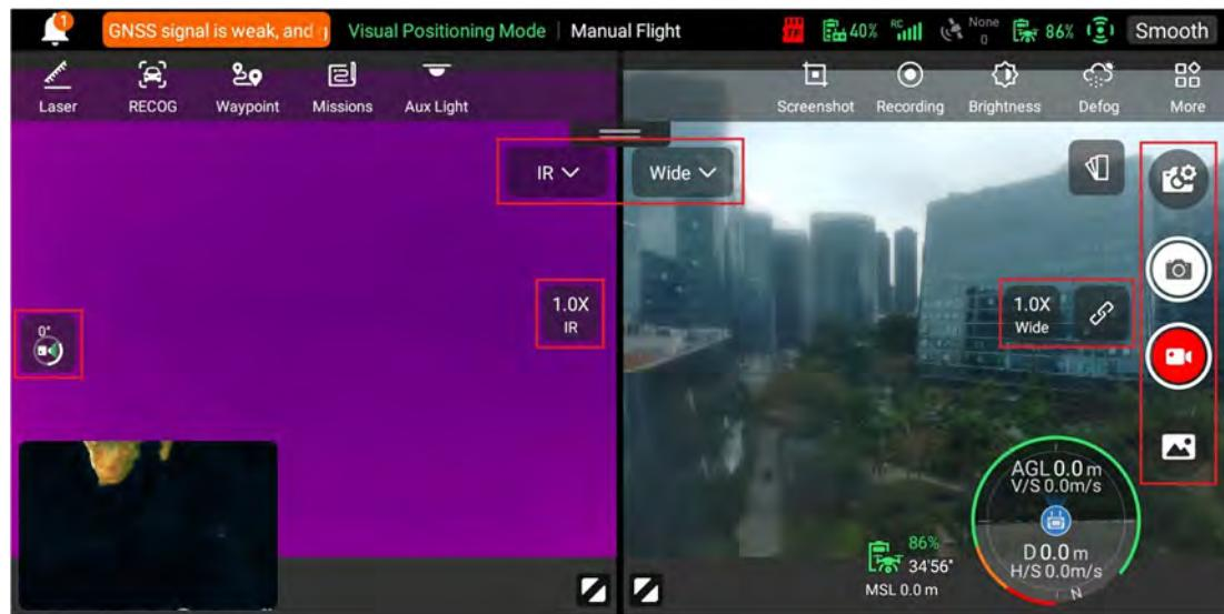
Fig 6-13 Camera Function Area (EVO Lite 640T Enterprise)
