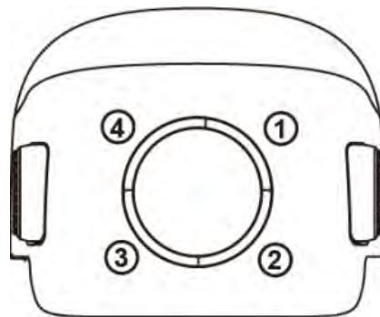
**Fig 5-4** Distribution of Battery Level Indicator
