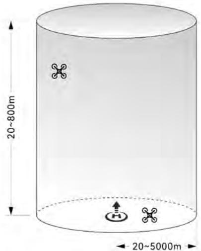
**Fig 2-2** Altitude and Distance Limitation Diagram
