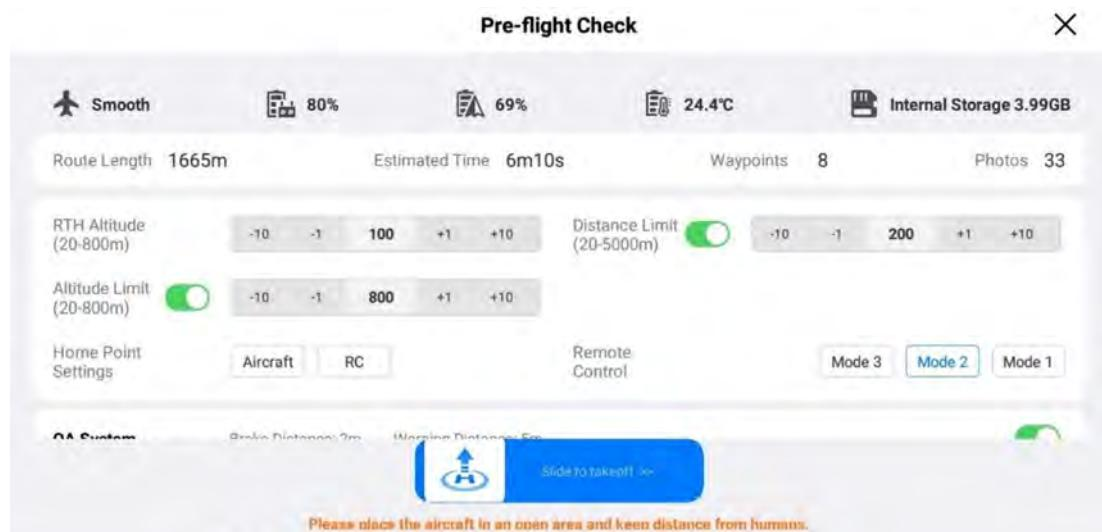
Fig 6-18 Pre-flight Check for a Flight Mission
