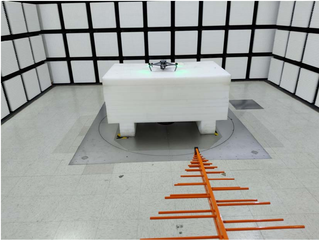
Radiated Emission 9 kHz-30 MHz Parallel View
