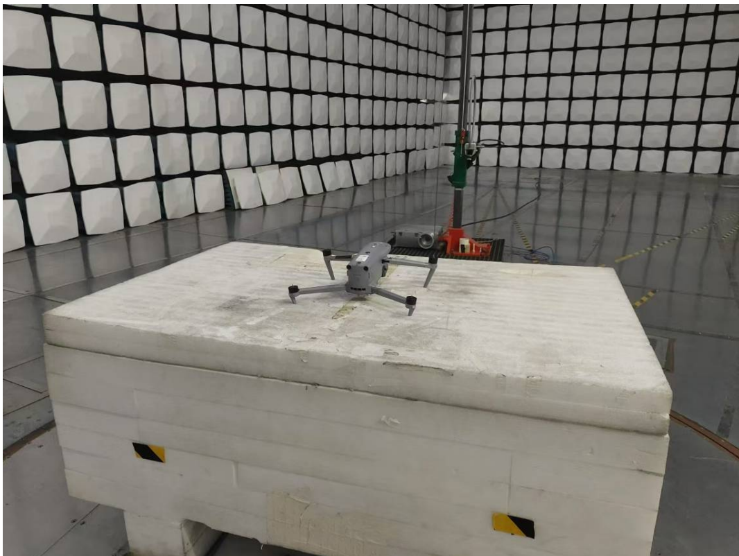
Radiated Emission 9k-30MHz Perpendicular View
