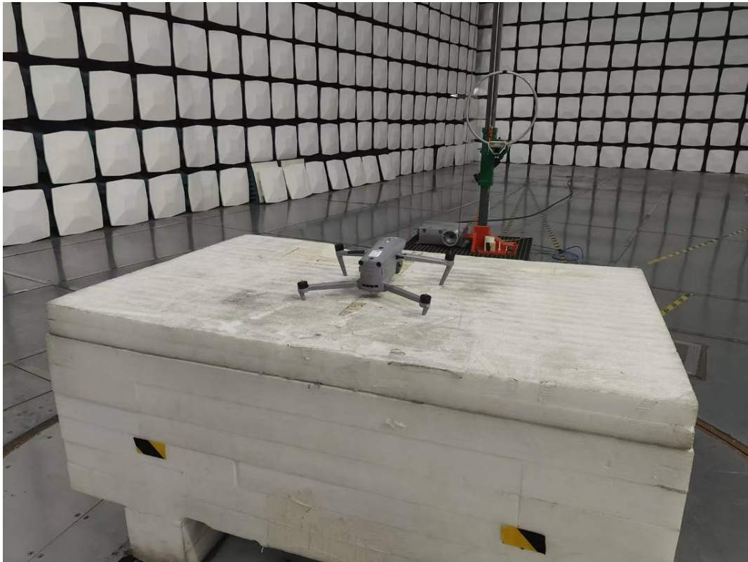
Radiated Emission 9k-30MHz Perpendicular View
