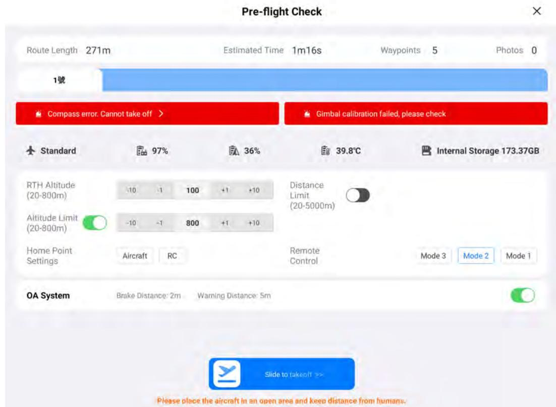
Fig 6-11 Pre-flight Check for a Flight Mission
