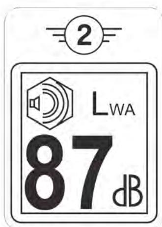
**Fig 3-17 A-weighted sound power level of the aircraft**
