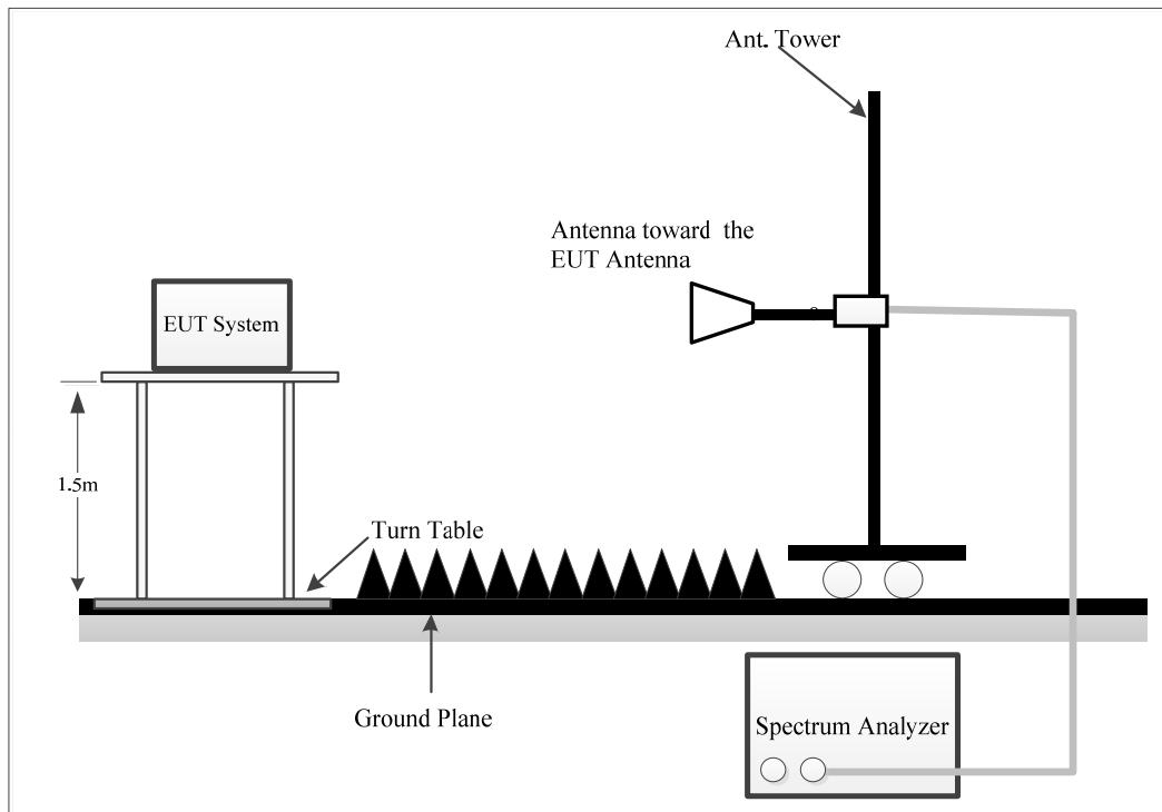
Place the measurement antenna in the main beam of the EUT then maximize the fundamental emission, noting that multiple peaks can be found at different beam orientations and/or polarizations.
