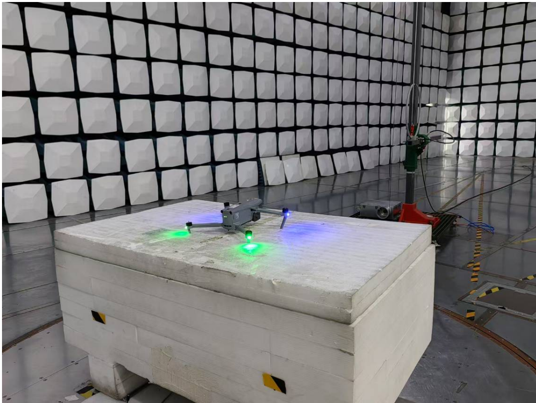
Radiated Emission 9k-30MHz Perpendicular View
