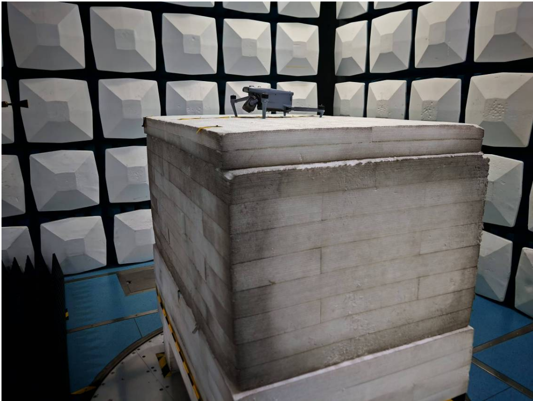
Radiated Emission 60-90GHz View
